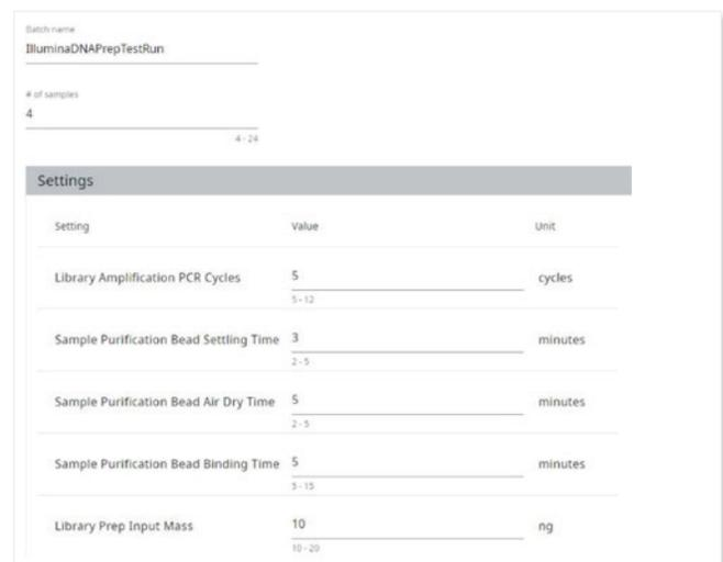
**Figure 2b. Configuration Run Screen:** Configuration Run screen allows users to define settings (e.g., number of samples, volumes, input concentrations) for a batch run. Sample data can be entered in .csv format.
