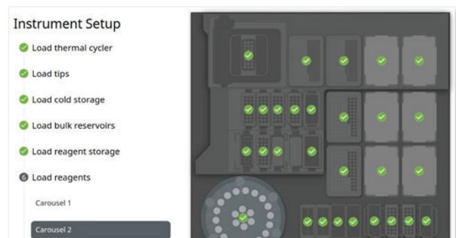
**Figure 3b. Deck setup:** A step-by-step series of prompts is directed by the application with the Dynamic DeckOptix system confirming correct labware placement while advancing steps through to completion in real-time.
