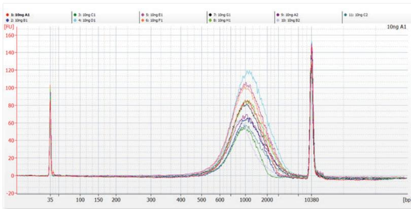
Figure 4: Bioanalyzer traces from the libraries prepared on Biomek NGenius system 10 ng run.
